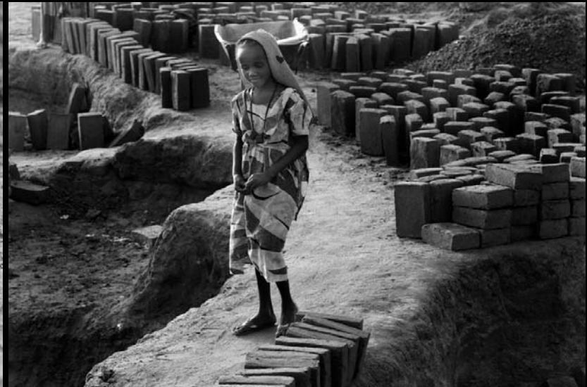
One standard room in the camp is usually 2m x 3m, requiring 1,000 bricks. A woman can make an average of 100 bricks a day. These mud bricks are an environmentally friendly alternative to the more common red bricks, which need to be fired. However they are not as durable.
